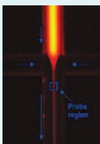
A 5 s integrated CCD image of Jurkat cells labeled with Calcein undergoing hydrodynamic focusing for high sensitivity detection.
